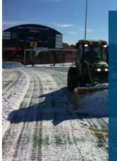
We use the Turf Pusher with our M6060 Kubota on natural and synthetic fields. It cuts plowing time by 50%. The biggest benefit is how safe the Turf Pusher is for the surface. We no longer worry about messing up and digging into a field as we did with the previous methods. It doesn't seem to move the crumb rubber around as much, which is great.
