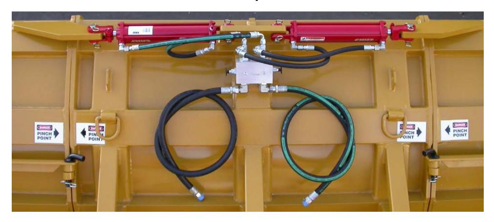
Install third valve hydraulic kit as shown
